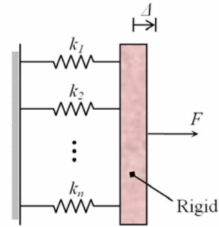
Figure 3:  $n$  springs in parallel.
