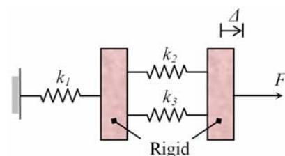
Figure 5: Parallel-series spring system.
