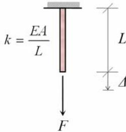
Figure 2: Hanger (bar) under load.
